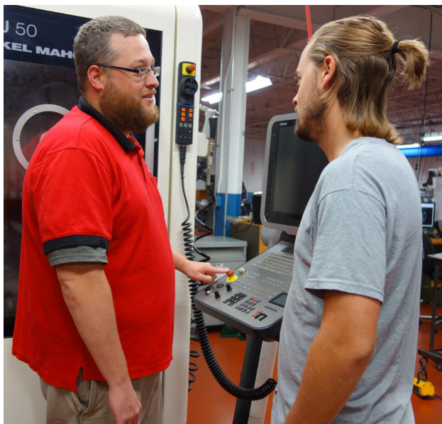
Doug Kuhn, Engineering Manager and Nate Kuhn, Assistant Foreman, get the DMU 50 five axes milling machine operational after their facility move.
